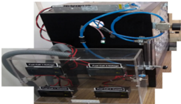
Fig. 4 Proton exchange membrane fuel cell system
