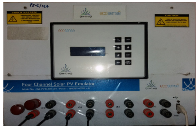
Fig. 2 Solar PV emulator
