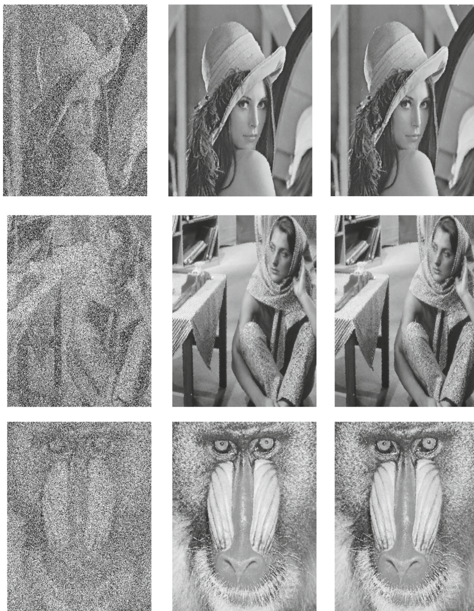
Fig. 6 Restoration of the Lena image, Baboon image, and Barbara image by the modified PRP method and the normal PRP method. From left to right: a noisy image with 55% salt-and-pepper noise and restorations obtained by minimizing z with the normal PRP method and modified PRP method
