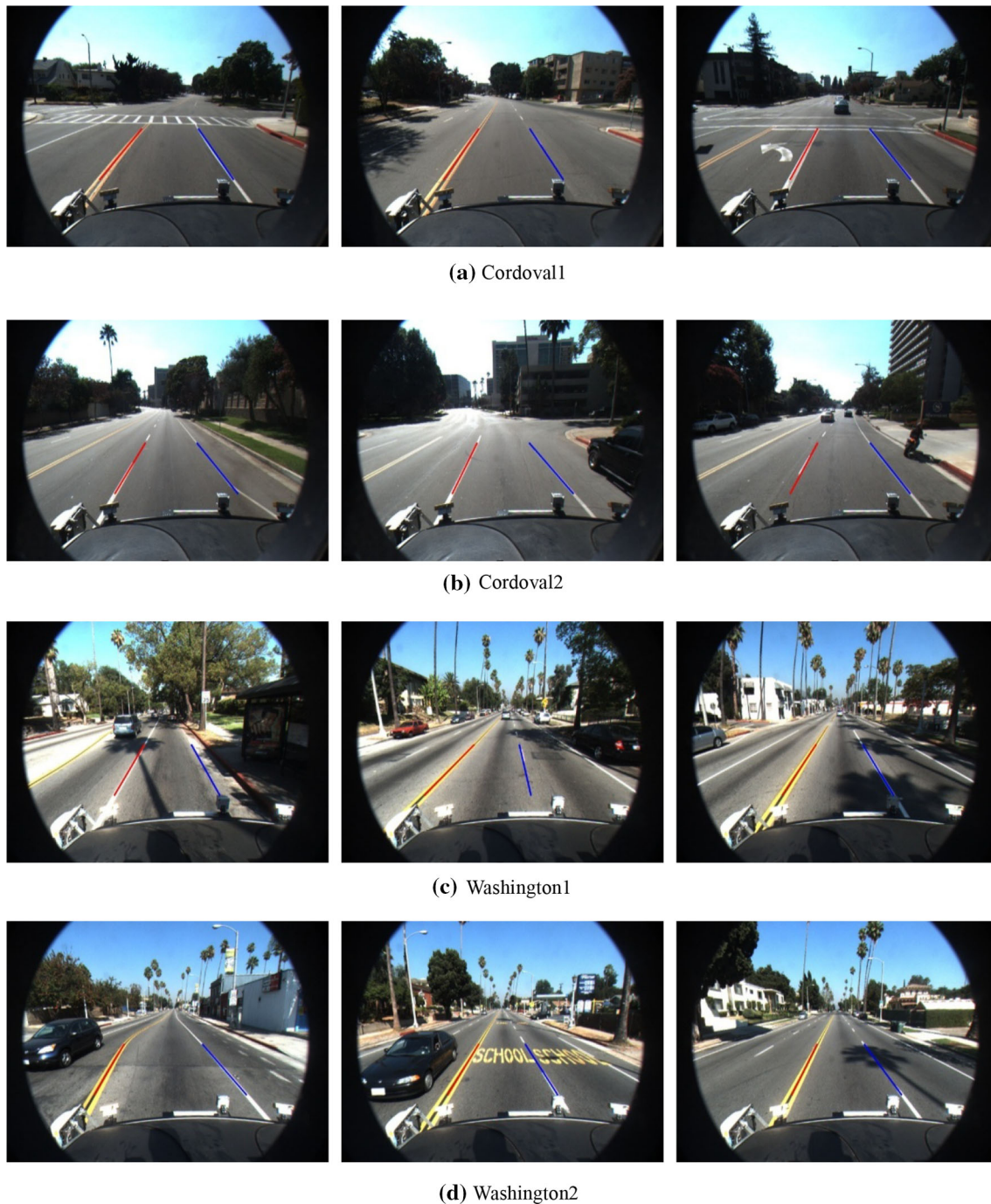
Fig. 14 Correct lane detection results
