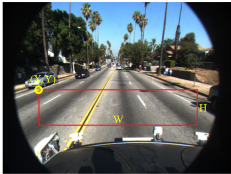
Fig. 2 The predetermined ROI, W is the width, H is the height, the units of X, Y, W and H are pixels
