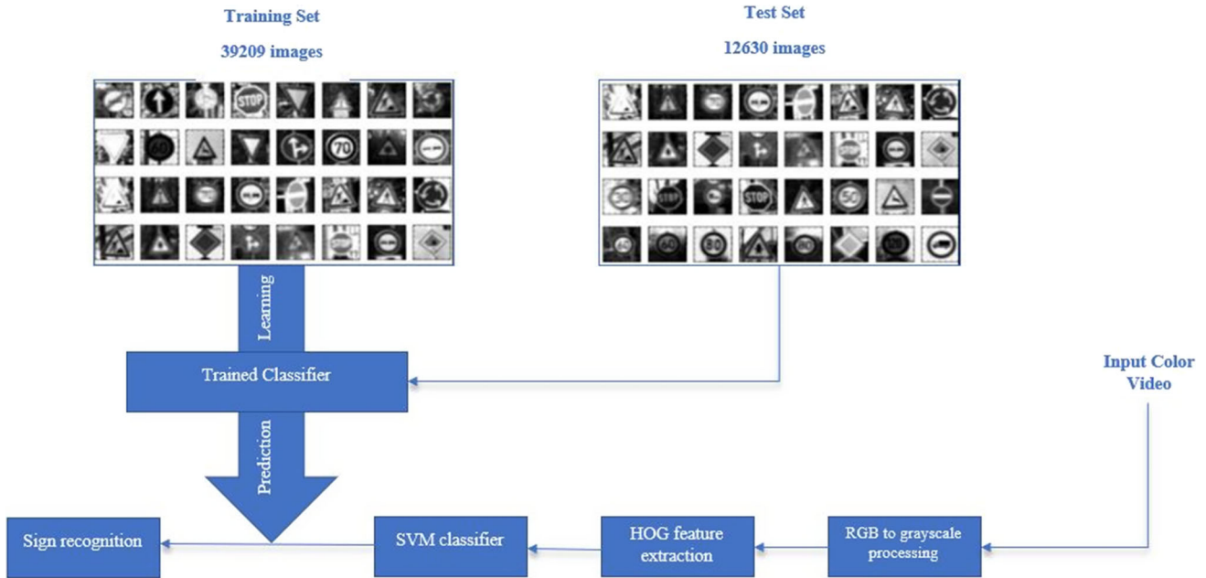
Fig. 3 The proposed system for the detection and classification of road signs
