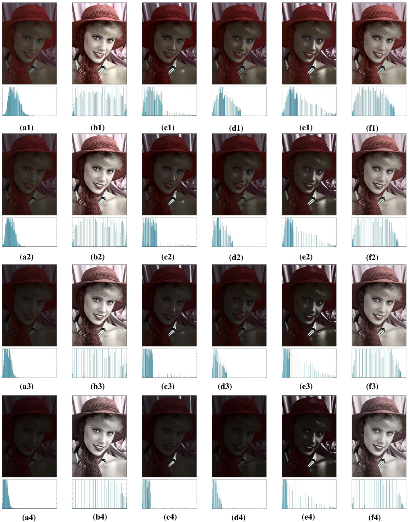
Fig. 7 'Woman' image and corresponding histograms at exposure levels 2, 3, 4, 5 in consecutive rows. a Test image and its enhanced versions using algorithms, b HE, c MMBEBHE, d BPDFHE, e MMSICHE, f FuzzyCIE
