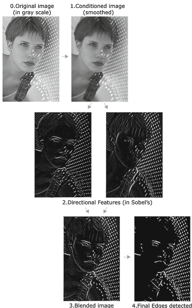
Fig. 2 Four sequential phases of edge detection using Sobel operator
