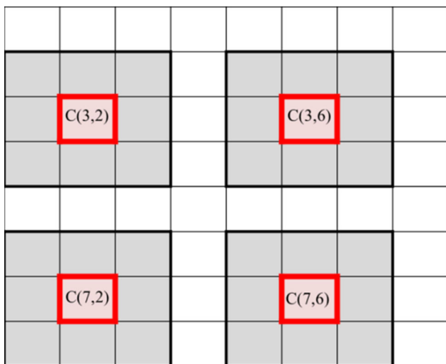
Fig. 3 Position of insertion four watermark bit ( c_{3,2} , c_{3,6} , c_{7,2} and c_{7,6} ) and their neighboring area (gray color) in a 8 \times 8 block
