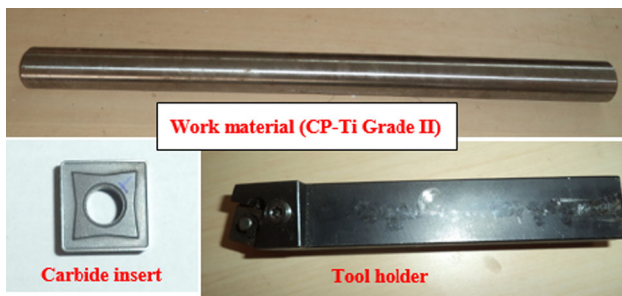
Fig. 1 Photographic view of workpiece, cutting insert and tool holder
