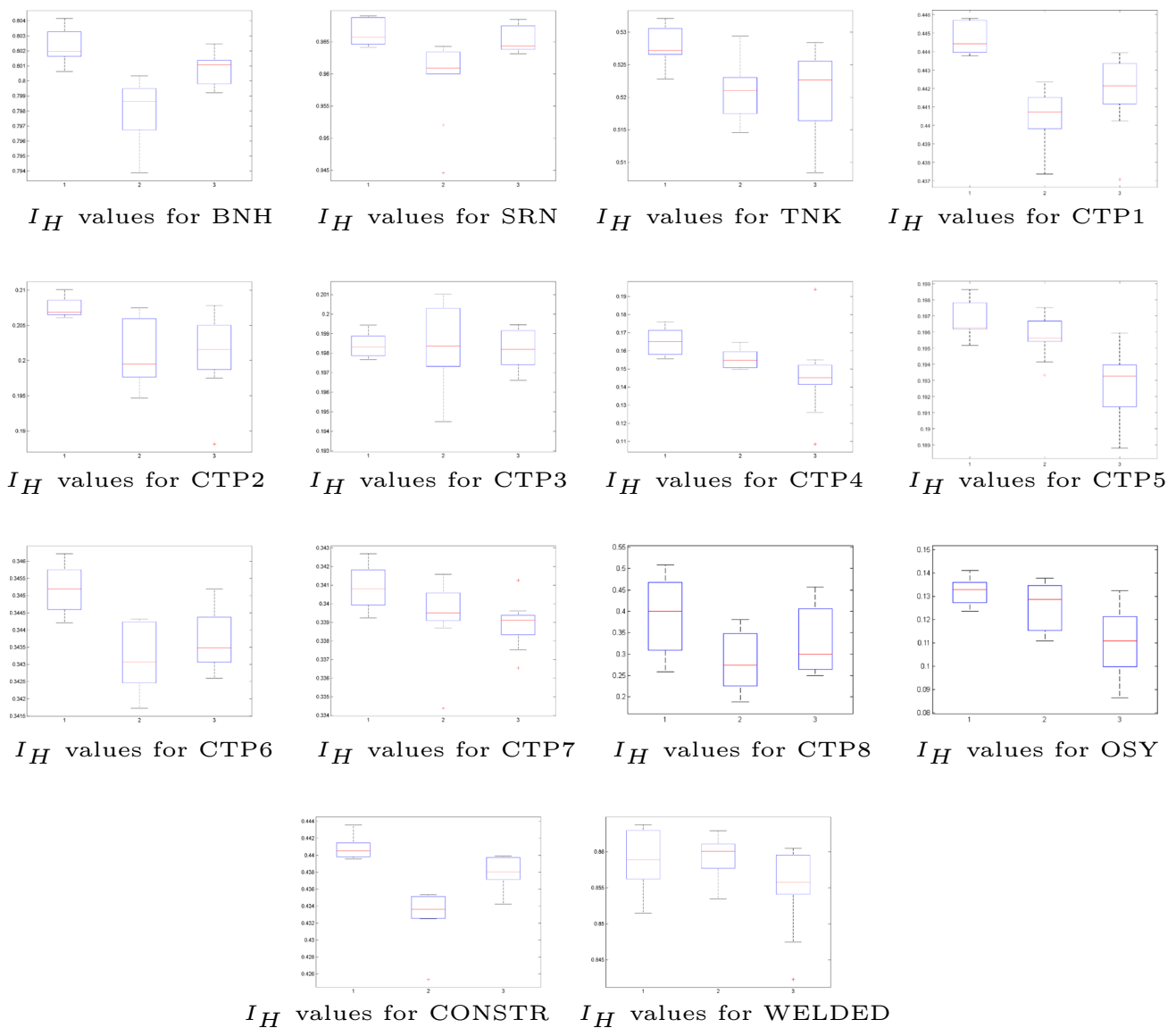
Fig. 12 Box plot of hyper-volume indicator ( I_H values) for all test functions by algorithms 1-3 represented (in order): the Proposed algorithm, Woldesenbet's, and NSGA-II
