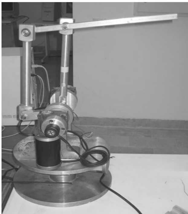
Fig. 5 A typical five-bar-linkage manipulator
