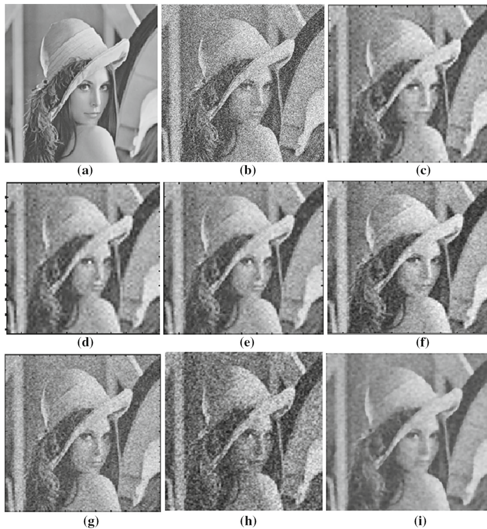
Fig. 4 a Original image, b noisy image, c Bayes Shrink, d Visu Shrink, e SURE Shrink, f bilateral filter, g Lee filter, h Kuan filter and i the proposed filter
