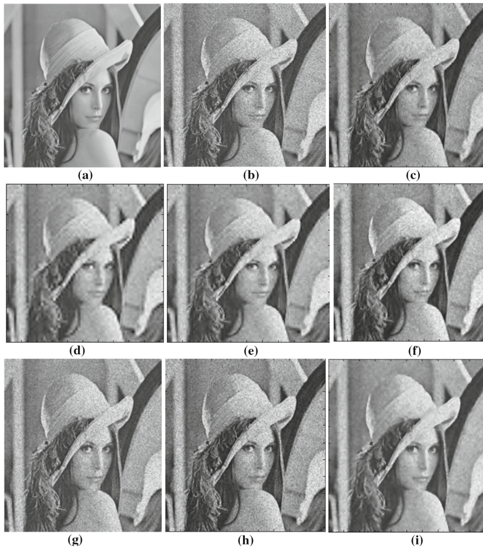
Fig. 9 a Original image, b noisy image, c Bayes Shrink, d Visu Shrink, e SURE Shrink, f bilateral filter, g Lee filter, h Kuan filter and the i proposed filter
