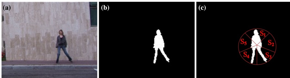
Fig. 2 a Original image, b silhouette image extracted by our proposed method based on IT2FLS, c silhouette slice partitions
