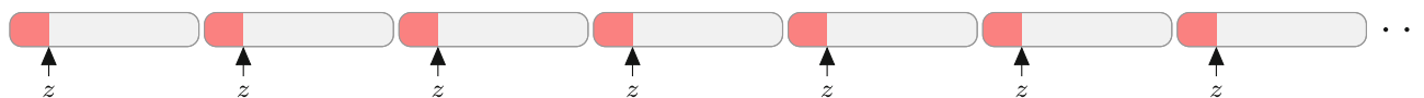
Fig. 1 Sketch of the function LOLZ. The red area indicates the region where leading ones and leading zeros are treated symmetrically
