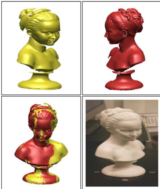
Fig. 1 From left to right. First row corresponds to two range images of the Cleopatra’s bust taken by a range scanner from two different points of view. Second row depicts the alignment achieved and the photo of the bust taken with a conventional CCD digital camera
