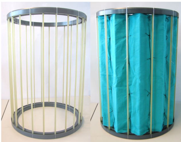
Fig. 1 Air gap spacer without and with draped fabrics
