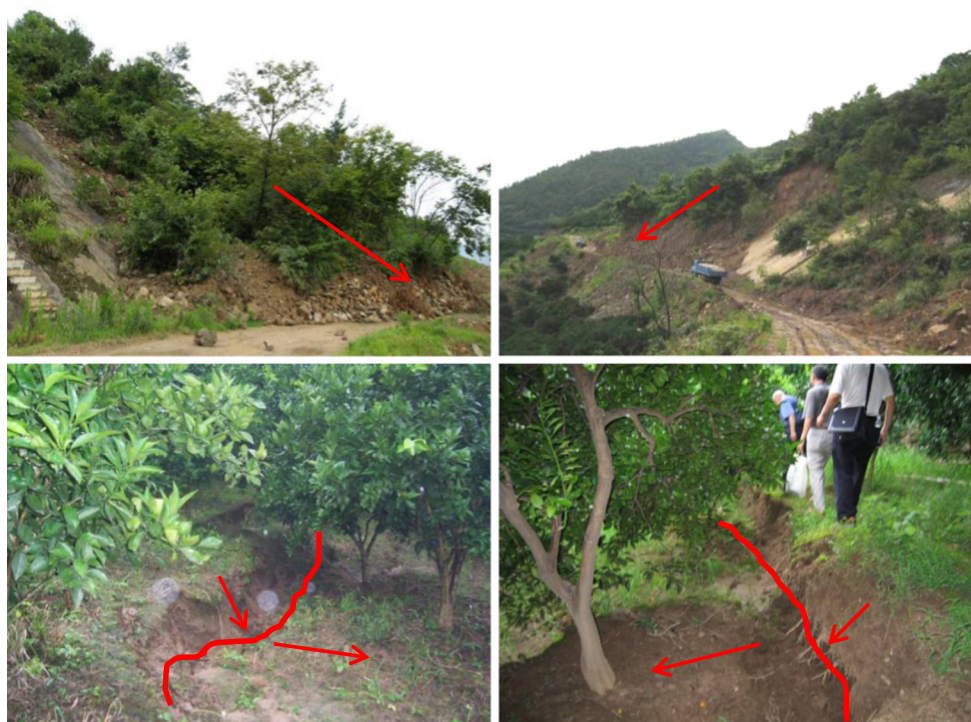
Fig. 6 Macroscopic deformation of Baishuihe landslide
