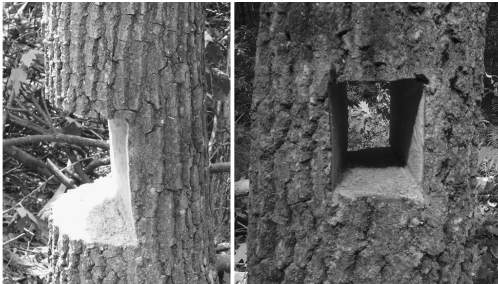
Fig. 3 Two examples of voids sawn through trees; trees were pulled to the left
