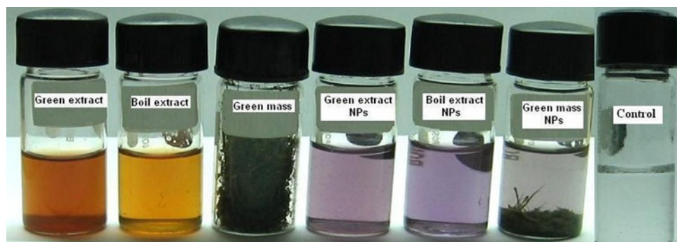
Fig. 2 Appearances of the green extract, boiled extract and green biomass used for reduction of 10^{-4} M \text{HAuCl}_4 and the change in color after the reaction and formation of gold NPs. No change in color in control with 10^{-4} M \text{HAuCl}_4
