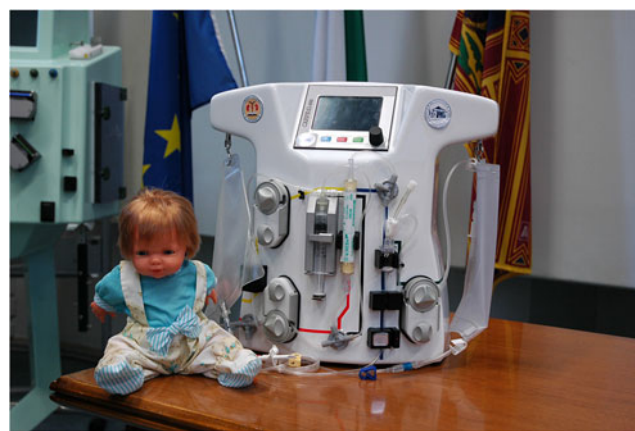
Fig. 3 The C ardio- R enal, P ediatric D ialysis E mergency M achine (CARPEDIEM) measures 44 (L) × 43 (H) × 23 (W) cm, weighs 13 kg, and is specifically designed as a miniaturized, transportable device
