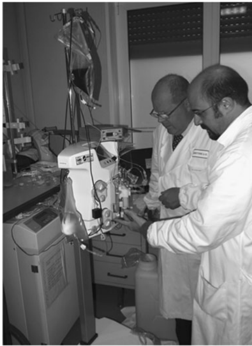
Fig. 4 The first in vitro trial of the CARPEDIEM machine. In this image the machine was running through a 4-French bilumen catheter
