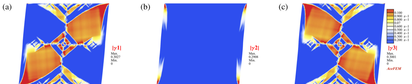
Fig. 15 Simple shear in case of orientation \omega = \pi/4 calculated by the rate-dependent algorithm (RD) with exponent r = 150 for FE mesh 100 \times 100 and maximum simple shear increment \Delta\bar{\gamma}_{12\max} = 10^{-3} . Slip-systems shear a |\gamma^1| , b |\gamma^2| and c |\gamma^3| for final strain \bar{\epsilon}_{12} = 0.05
