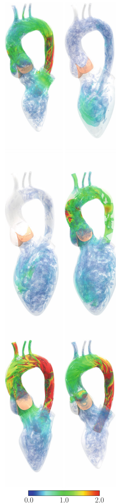
Fig. 22 Isosurfaces corresponding to a positive value of the second invariant of the velocity gradient tensor, colored by the velocity magnitude (m/s). The frames are for the same instants as in Fig. 19
