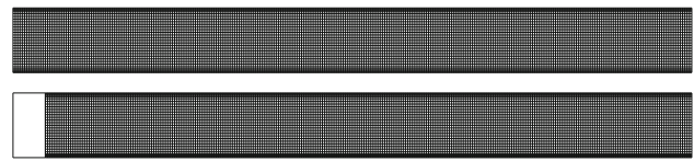
Fig. 3 Meshes for the OS (top) and CFP (bottom). The lines are the element boundaries. Except for the part of the domain where the CFP mesh has only one element, the two meshes have identical refinements
