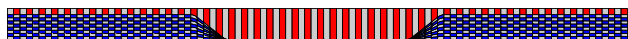
Fig. 7 Mesh-1-reduced. At the center part, the blue–gray elements collapse to the SI, and only the special quadratic NURBS elements remain, expanding to the SI. The checkerboard coloring is for differentiating between the NURBS elements. (Color figure online)
