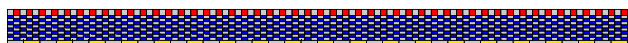
Fig. 5 Mesh-1. The yellow–gray elements, which are between the SI and the bottom solid surface, will collapse. The red–gray elements are the special quadratic NURBS elements we want to be left with, and they are placed at the top. The checkerboard coloring is for differentiating between the NURBS elements. (Color figure online)
