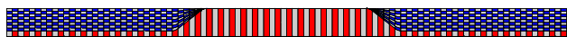
Fig. 8 Mesh-2-reduced. At the center part, the blue–gray elements collapse to the top solid surface, and only the special quadratic NURBS elements remain, expanding to the top solid surface. The checkerboard coloring is for differentiating between the NURBS elements. (Color figure online)
