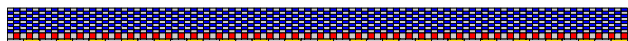
Fig. 6 Mesh-2. The yellow–gray elements, which are between the SI and the bottom solid surface, will collapse. The red–gray elements are the special quadratic NURBS elements we want to be left with, and they are placed just above the SI. The checkerboard coloring is for differentiating between the NURBS elements. (Color figure online)
