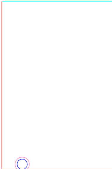
Fig. 11 A 2D tire model with grooves. Computational domain and boundary conditions. The left ( red ) and bottom ( yellow ) boundaries are the inflow and the moving planar surface, where the velocity is U_0 . The innermost ( blue ) circle is the spinning surface, where the velocity is U . The larger ( pink ) circle is the SI. The bottom of the SI is coinciding with the planar surface and the interface of the spinning and planar surfaces. The conditions at the right ( green ) and upper ( cyan ) boundaries are stress-free and slip, respectively. (Color figure online)
