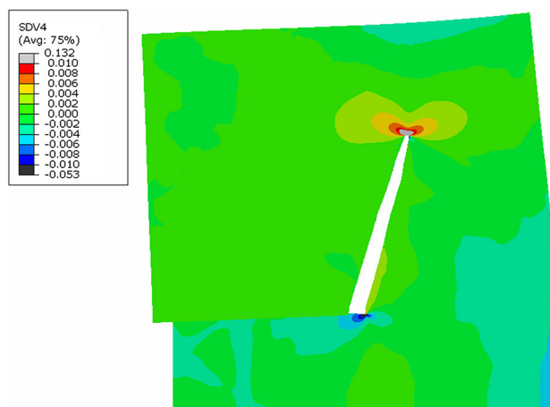
Fig. 6 A post-processed plot of deformation at t = 75 us. The displacements have been scaled by a factor of 5 and areas of model where d > 0.99 have been removed from the plot to show cracks. The contour of strain component \epsilon_{11} is shown
