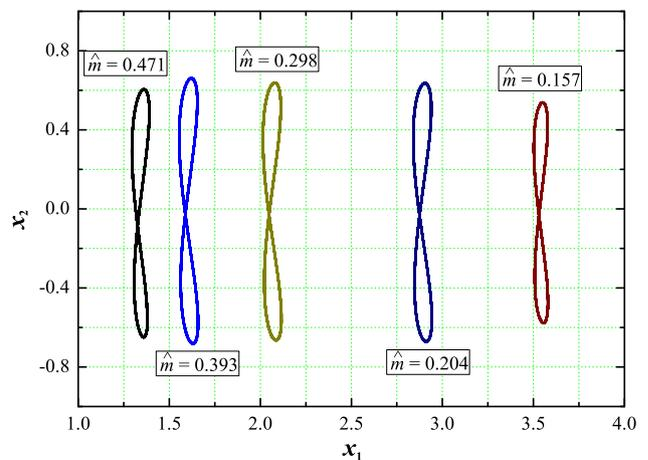
Fig. 15 8-Profile trajectory of the oscillating circular cylinder at different  $\hat{m}$ .
