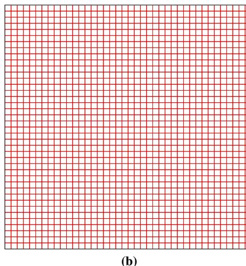
Fig. 5 The lid-driven cavity flow. **a** Schematic view. **b** Finite element mesh
