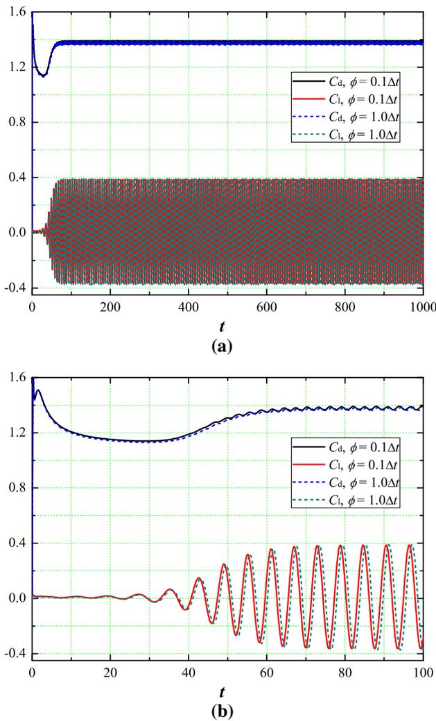
**Fig. 9** Time history of drag and lift coefficients. **a** Full-size view. **b** Zoom-in view
