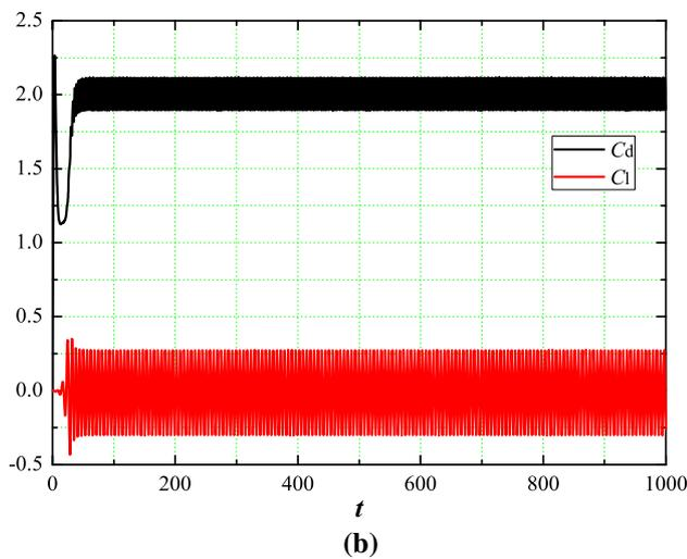
Fig. 13 Time history of aerodynamic parameters at  $\hat{m} = 0.408$ . **a** Cylinder displacement. **b** Fluid force coefficients
