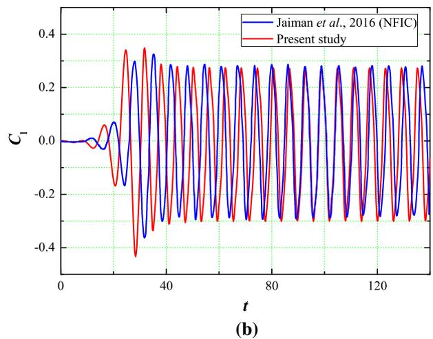
Fig. 14 Time history of lift coefficient at  $\hat{m} = 0.408$
