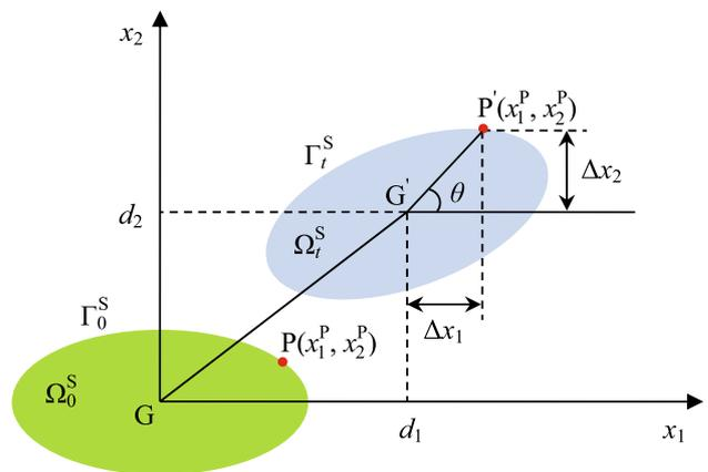
Fig. 4 Schematic view of the generalized planar rigid-body motion
