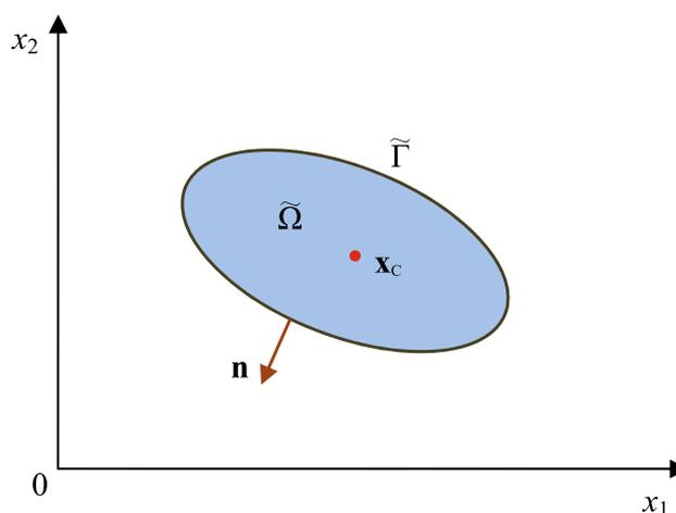
Fig. 1 Illustration of a generic smoothing cell for an arbitrary point
