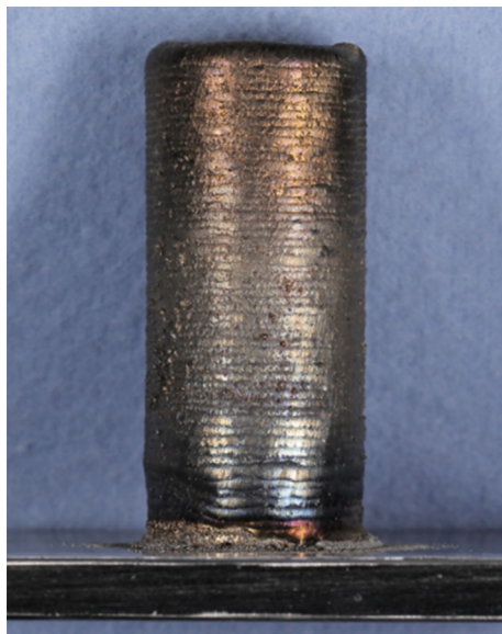
Fig. 1 Side view of as-built 304L LENS tube. The individual layers are clearly visible, as well as some discoloration due to the heat up of the tube during the build. The tube had a 50 mm height, 16 mm inside diameter, and 24 mm outside diameter
