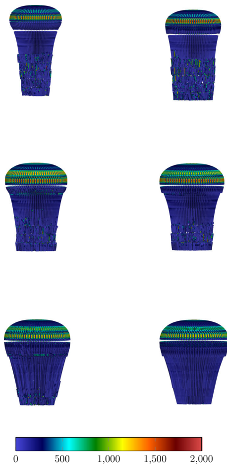
Fig. 5 Single MP parachute maximum principal fabric stress (lb/in 2 ) during Stage 1 to 2 disreef at 0.5 s intervals
