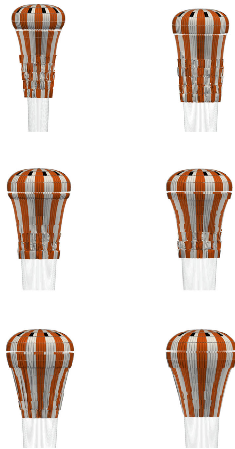
Fig. 4 Single MP parachute during Stage 1 to 2 disreef at 0.5 s intervals
