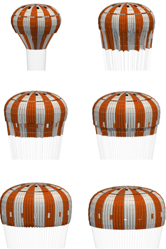
Fig. 10 Single MP parachute during Stage 2 to 3 disreef at 0.5 s intervals
