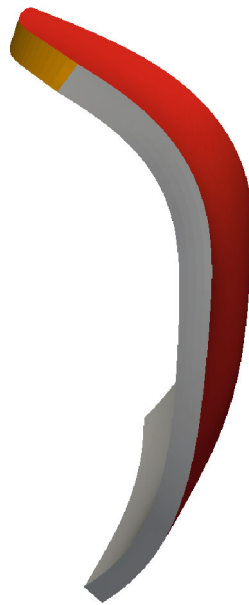
Fig. 28 A curved tube. Opening-angle comparison for the cutting location \phi_c = \pi/2 , for the case \phi = \pi/2 and \lambda_z = 1.2
