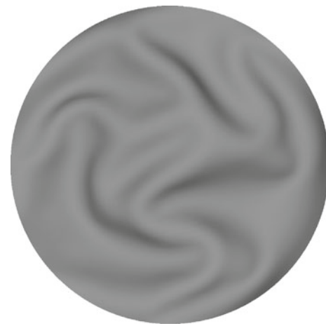
Fig. 3 Top view of the membrane deformed configuration at t = 0.15 s. Despite the complex deformation pattern, the wrinkles on the membrane surface are smooth
