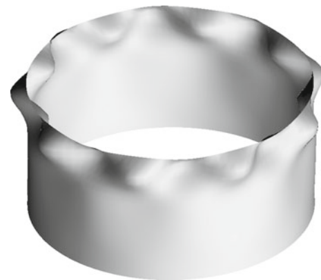
Fig. 10 First buckling mode of the compressed simply supported cylindrical shell with metal outer surface and ceramic inner surface ( n = 1 )
