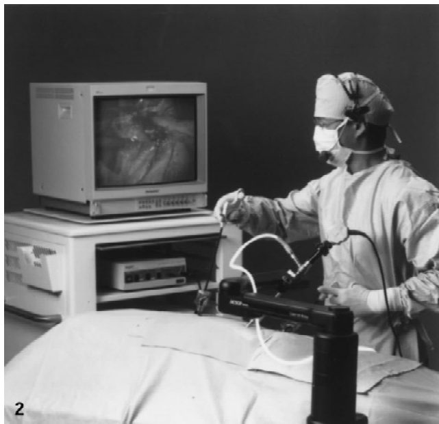
Fig. 2. Voice control interface in use with the AESOP robot. (Photo courtesy of Computer Motion)
