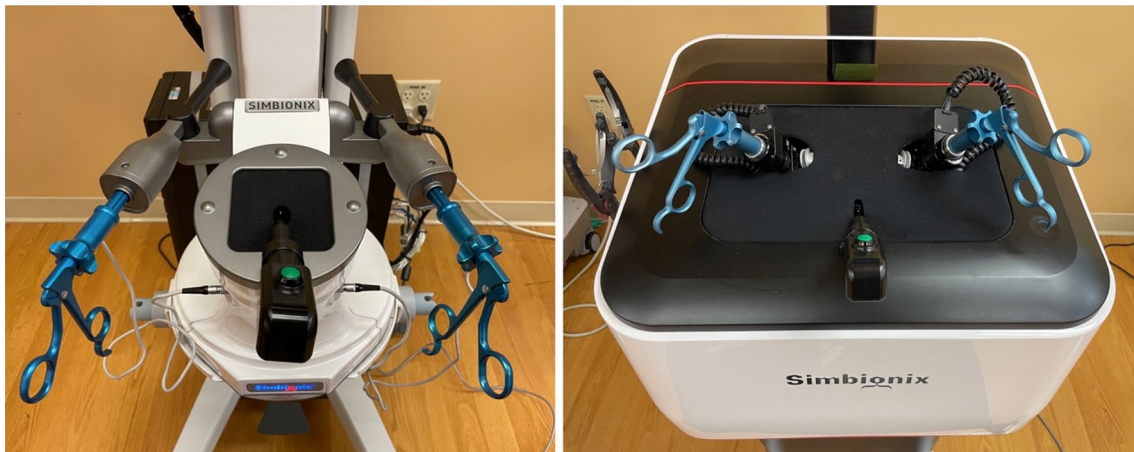
Fig. 2 Surgical interface for the haptic (right panel) LAP Mentor III and nonhaptic (left panel) LAP Mentor Express simulators. The added bulk of the haptic platform's interface is required to accommo-
