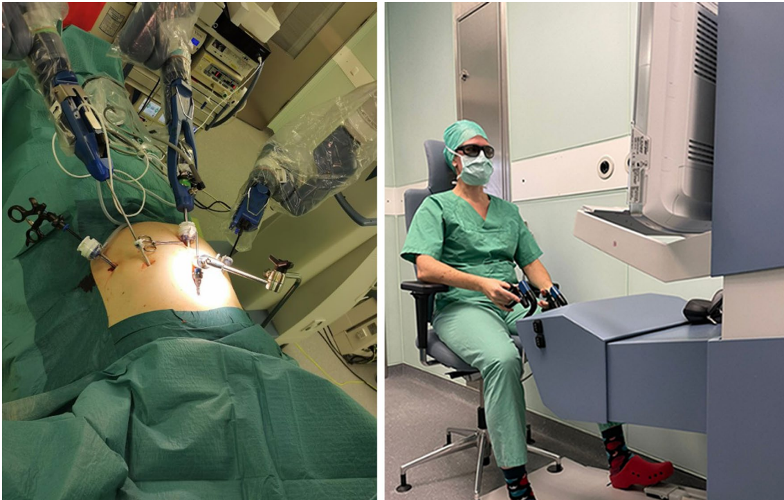
Fig. 3 Real life situation of the connected intracorporeal Senhance® system with 3 arms: the camera in the middle, the Johan Grasper in the left upper quadrant and the ultracision device on the right upper abdomen, as well as the surgeon at the cockpit
