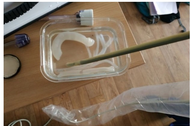
Fig. 4 Recording of the ultrasound images on the agar model using a laparoscopic ultrasound probe
