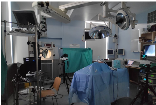
Fig. 1 Photography of the experimental setup of a porcine cadaveric laparoscopic model in a dedicated research theatre with schlieren optical imaging system with one (of a pair) 40 cm parabolic mirror (far left) Canon 5D mk III camera with EF 100 mm f/2.8 lens (left) and laser light source (far right)
