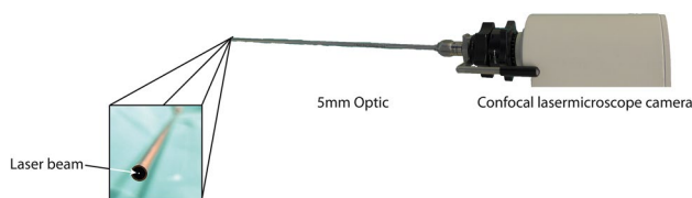
Fig. 1 Confocal laser microscope device for minimal-invasive approach. The CLM camera device is composed of a confocal laser scanning microscope device and rigid 5-mm endoscope with Hopkins-rod lenses
