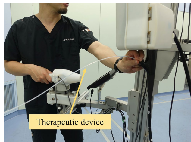
Fig. 7 While operating the handle of the robotic-assisted flexible endoscope with one hand, it is possible to simultaneously fine tune the position of therapeutic devices with the other hand stretched to the forceps channel
