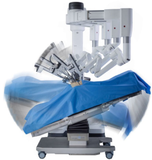
Fig. 1 Illustration of the da Vinci® Table Motion (dVTM) for the da Vinci Xi surgical system (Intuitive Surgical Inc., Sunnyvale, CA, USA). dVTM is a new feature comprising a unique operating table by Trumpf Medical Systems that communicates wirelessly with the da Vinci Xi. The da Vinci Xi surgical system and the TruSystem 7000dV operating table (TS7000dV, TRUMPF Medizin Systeme GmbH & Co. KG, Saalfeld, Germany)
