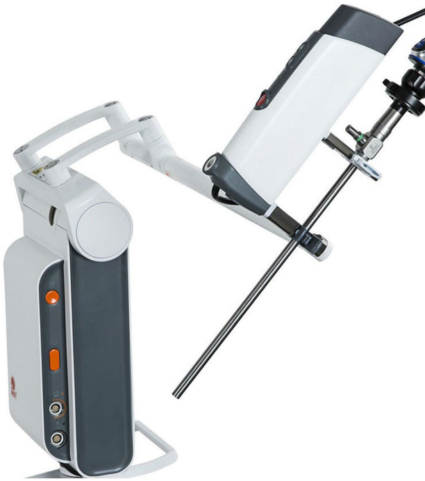
Fig. 2 Laparoscopic- and base unit of the AutoLap™ system
