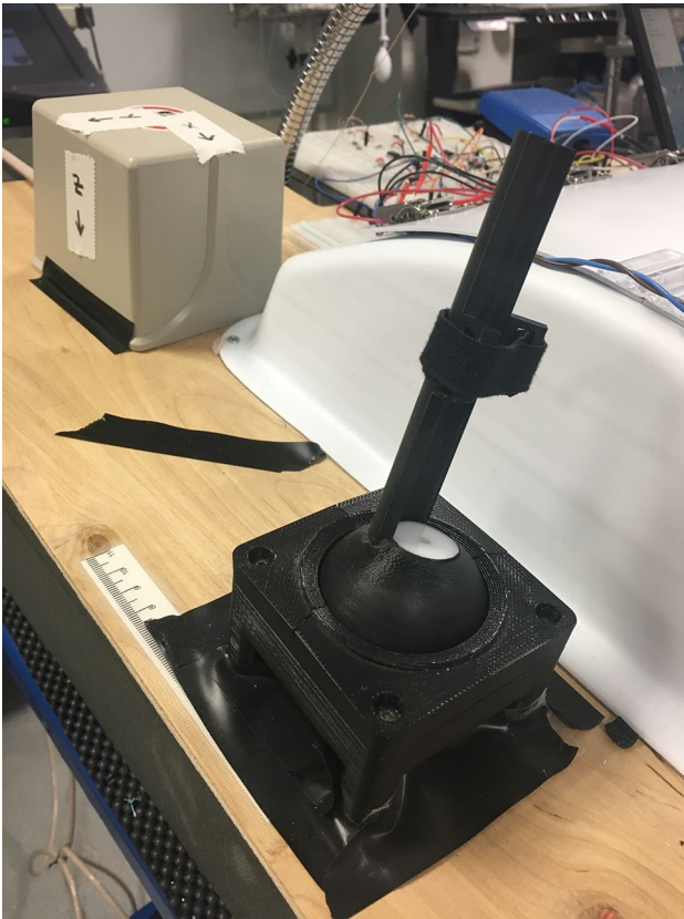
Fig. 4 The device used to calibrate the placement of the trakSTAR sensors on the instruments. During use, the tool tip is inserted into the white mount, and the tool shaft is strapped to the vertical portion, which can rotate to all angles via a spherical joint centered around the tool tip
