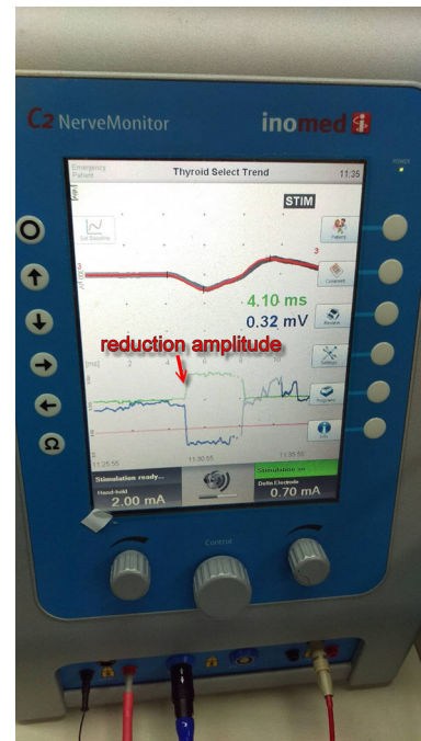
Fig. 5 One event in which >50% reduction in EMG amplitude and >10% increased nerve latency occurred; this improved after releasing the thyroid retractor (arrow)
