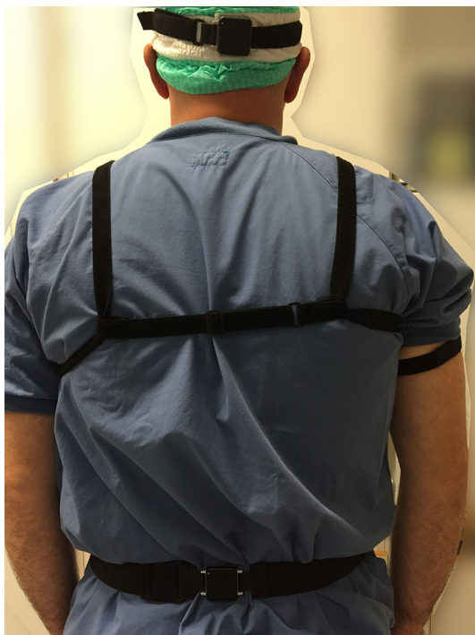
Fig. 2 Wearable wireless motion tracking sensors placed on the surgeon before the surgery
