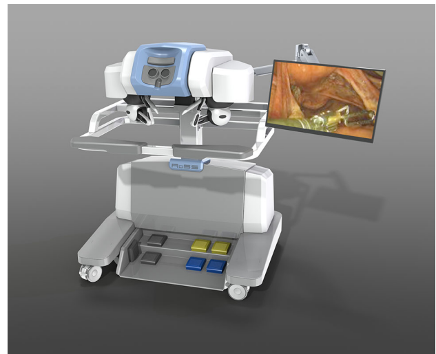
Fig. 1 The RoSS™ Robotic Surgery Simulator (Simulated Surgical Systems LLC, San Jose, CA, USA)
