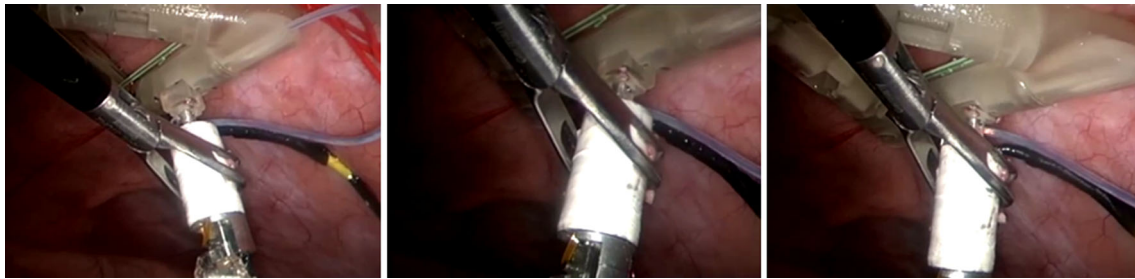
Fig. 8 Docking/undocking procedure: From left to right, the robotic module is moved close to the magnetic frame, the docking/undocking mechanism is opened, and the camera robot is anchored to the frame
