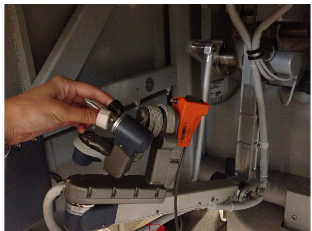
Fig. 2 da Vinci master handle augmented with a custom actuator for haptic display of instrument vibrations
