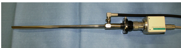
Fig. 1 CMOS camera mounted on 10 mm rigid scope with xenon light cable
