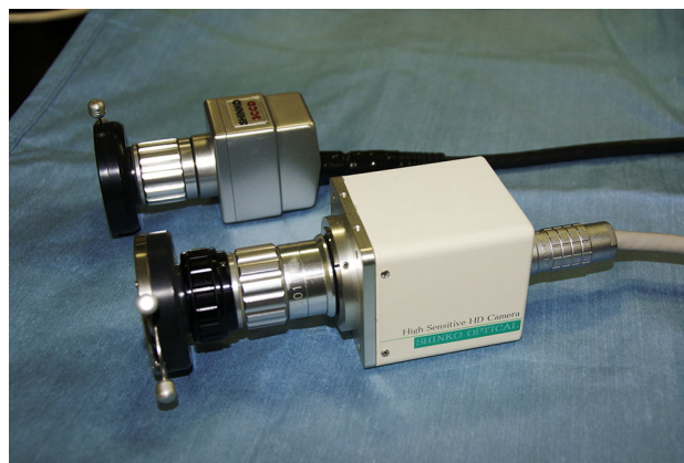
Fig. 3 Images of 3CCD/CMOS camera heads above : 3CCD camera head below : CMOS camera head
