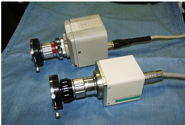
Fig. 5 Images of EM-CCD/CMOS camera heads above : EM-CCD camera head below : CMOS camera head
