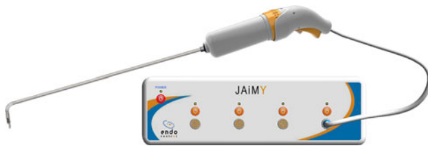
Fig. 4 Prototype of hand-held robotically controlled laparoscopic instruments (JAIMY, Endocontrol, Grenoble, France)
