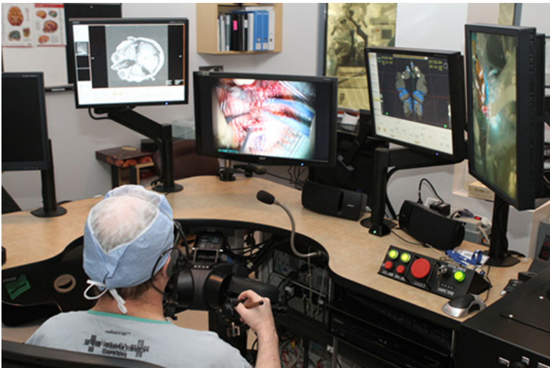
Fig. 8 NeuroArm controllers allow haptic feedback, three-dimensional visualization, an intuitive pencil-type interface, and the ability to visualize radiologic images with the operation (Calgary, AB)
