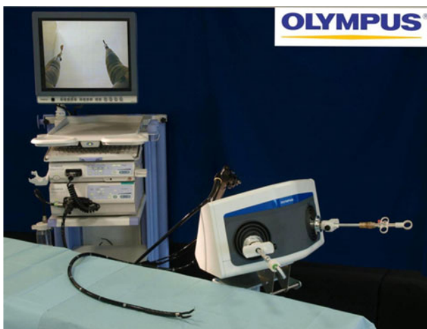
Fig. 1 The EndoSAMURAI™ system: a multitasking platform with a flexible endoscope attached to an ergonomic surgical manipulator workstation. The end-effectors can be manipulated via this workstation
