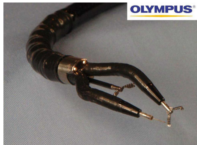
Fig. 2 Tip of the flexible endoscopic multitasking platform with two arms in triangulation for the manipulation of the end-effectors
