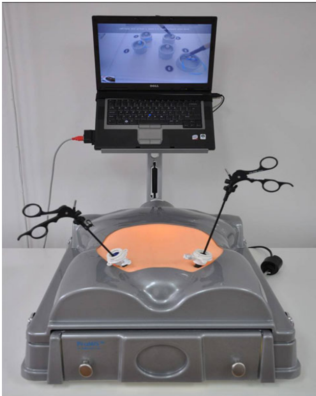
Fig. 2 The ProMIS augmented reality simulator
