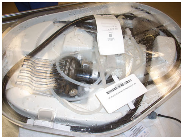
Fig. 6 Experimental processing of the GIF N-180 endoscope using a modified Y-adaptor linking parts of different Quick Connects in the C1140 Flexible Endoscope Processing Tray (not validated by Steris Inc.)
